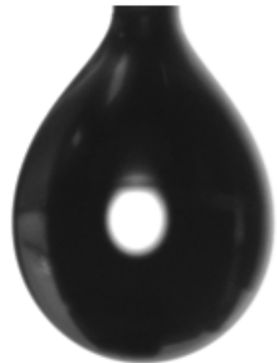
Figure 12: A typical fluidic pendant droplet generated using experimental apparatus
