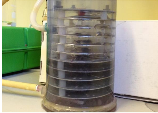
Figure 5: The new EC reactor.
